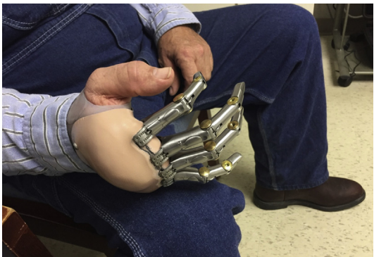
Fig. 10. At the MCP level, 4 Point Designs Point Digits are used to create a robust, heavy-duty prosthesis for this farmer. (Courtesy of Handspring Clinical Services, Middletown, NY; with permission.)
