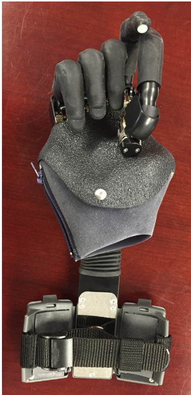
Fig. 19. A full 5-digit Össur i-Digits system used for a patient with amputation of all digits proximal to the MCPJs. (Courtesy of Handspring Clinical Services, Middletown, NY; with permission.)
