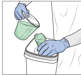
6. Fill mold with plaster or dental stone taking care to prevent expansion of the silicone with plaster bandage.
